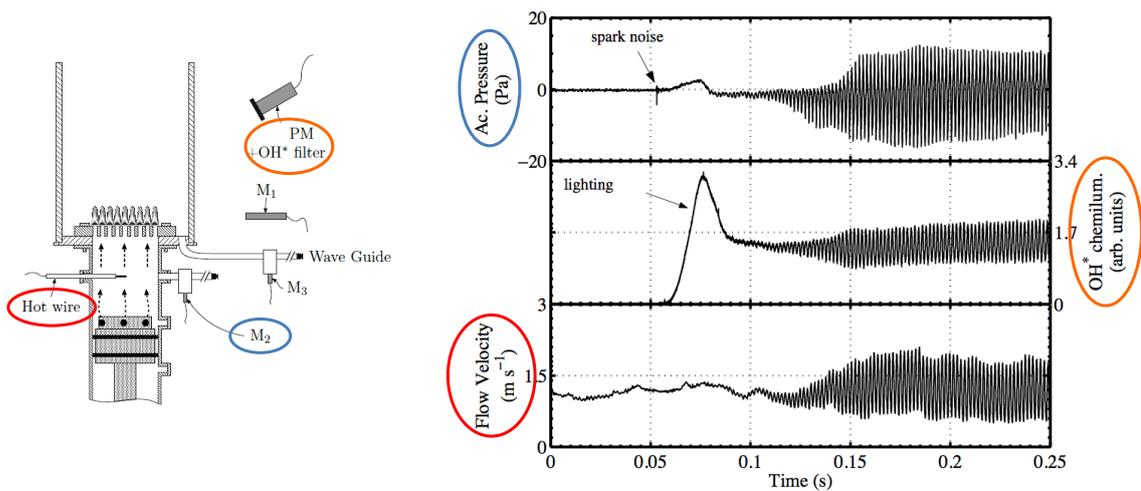
During unstable operation, after ignition and transient growth, oscillations of flow variables reach a limit cycle
