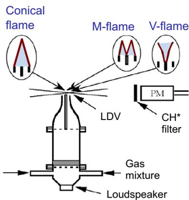
The flame can be stabilized in three different configurations. (film by Daniel Durox, EM2C)
