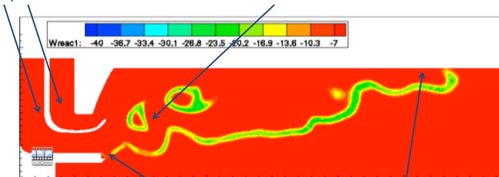
C. Anchoring devices used to stabilize the flame
