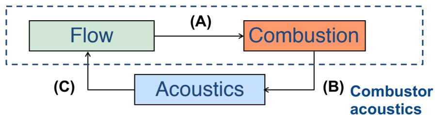
The objective is to decouple the analysis of flow and combustion dynamics (nonlinear problem) from the analysis of the combustor acoustics (linear problem).
