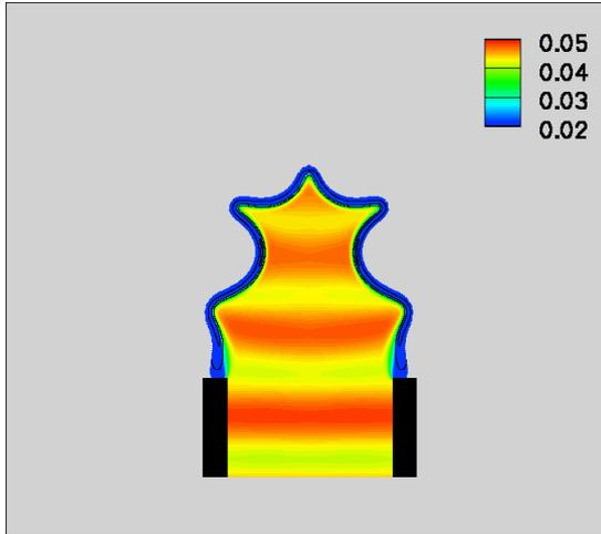
Conical flame perturbed by equivalence ratio modulations
