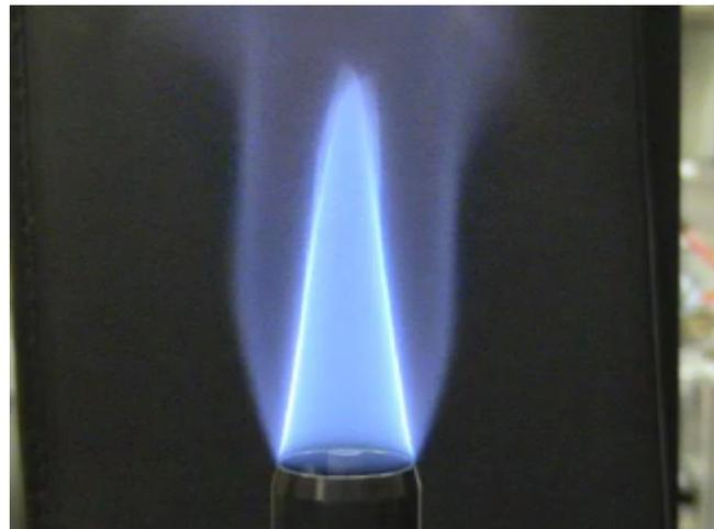
Experiments indicate that flames are sensitive to perturbations and that their response depends on the flame geometry, modulation frequency, type of perturbation and amplitude
