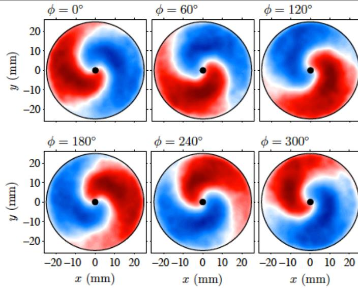
Figure 19: Phase-averaged images of the light intensity deviation from the mean distribution in the burner gathered from a top view at the interaction frequency (254 Hz).
