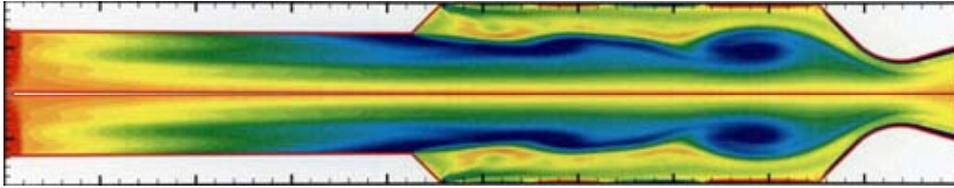
Resonant vortex shedding before control (elevated level of pressure fluctuation)
