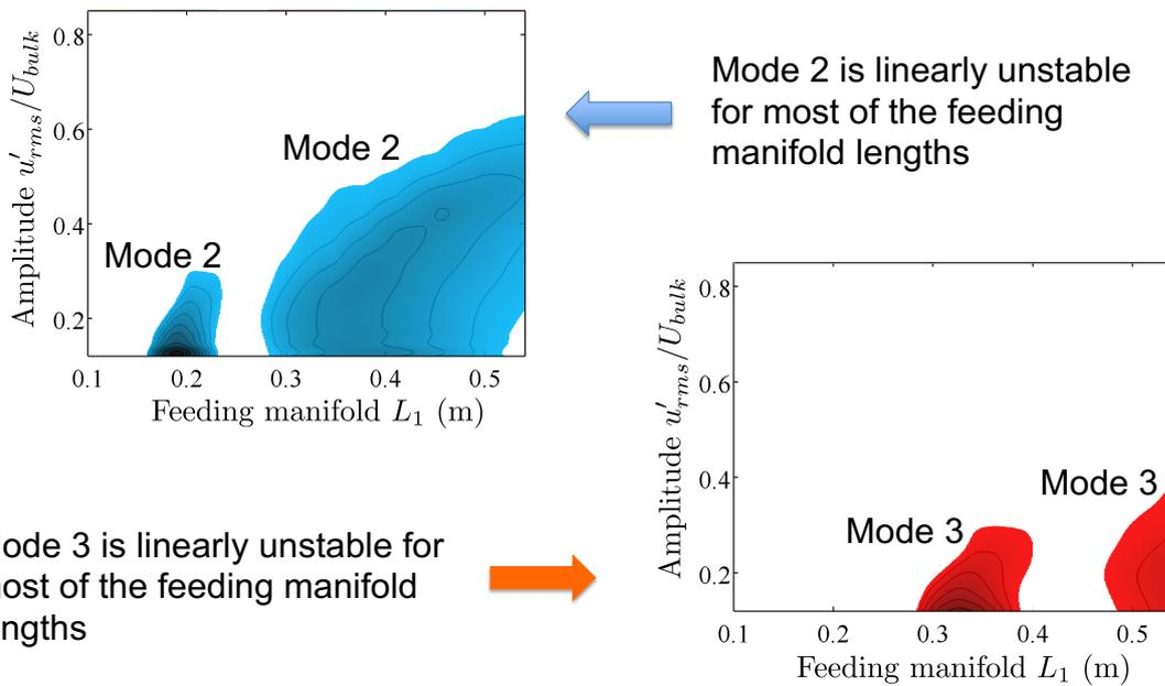
Mode 3 is linearly unstable for most of the feeding manifold lengths
