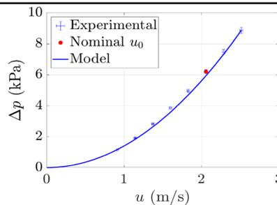
Pressure loss measurements in the SICCA-Spray burner as a function of the velocity at the hot-wire probe position. The value at the nominal operating conditions is indicated by a red dot
