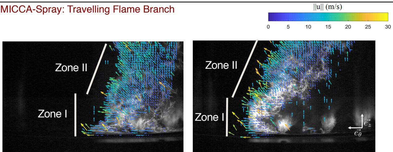
The volumetric expansion of the burned gases drives the movement of the flame.
