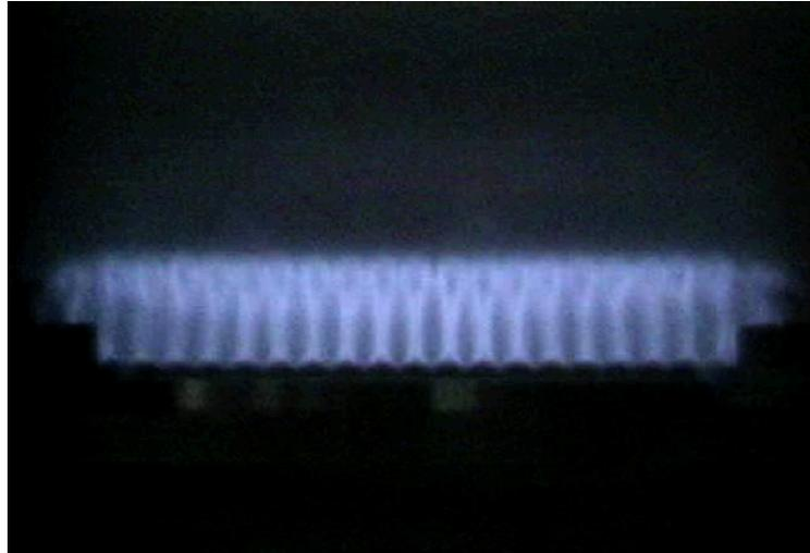
Oscillation cycle ( $f=530$  Hz) in a typical unstable situation (high amplitude sound radiation  $> 110$  dB at 40 cm from the burner)
