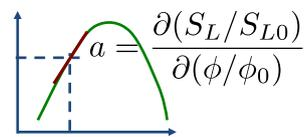
Heat release rate fluctuations result from fuel mass burning rate (function of  $\phi$  and mean flame surface area) and flame surface area fluctuations (function of  $\phi$ ,  $v$  and mean flame surface area).
