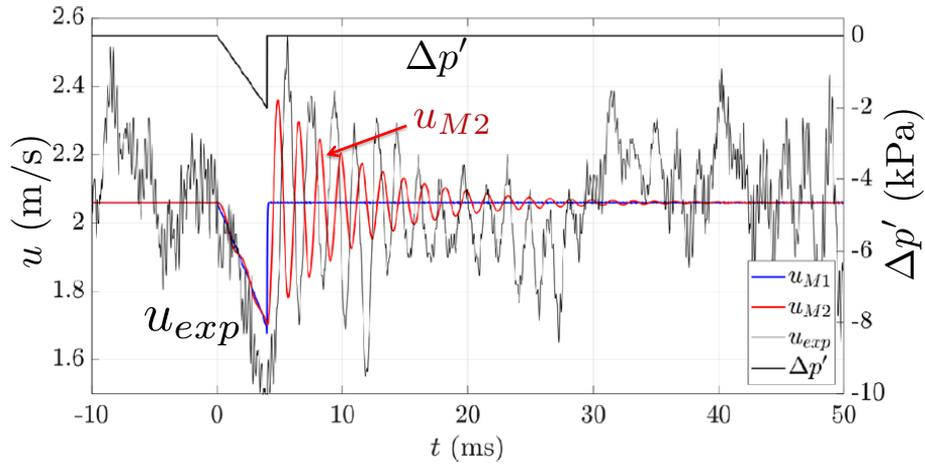
Velocity obtained at the hot wire position using model M1 (blue) and M2 (red). The velocity measured by the hot wire is shown as a thin black line. The pressure perturbation used for the present calculation is shown as a thicker black line on top, associated with the right axis.
