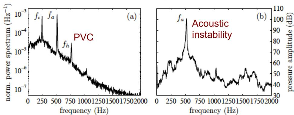
Figure 15: Spectral distributions of photomultiplier (a) and microphone (b) signals,  $\phi = 0.69$ ,  $u_b = 9.9 \text{ m.s}^{-1}$ . One vertical half of the photomultiplier's field of view is masked, and the signal has been normalized by the mean value. The microphone is located outside of the flame tube.  $f_i$ ,  $f_a$ , and  $f_h$  denote interaction, acoustic and helical-mode frequency, respectively.
