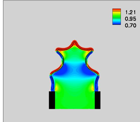
Velocity field perturbed by equivalence ratio modulations
