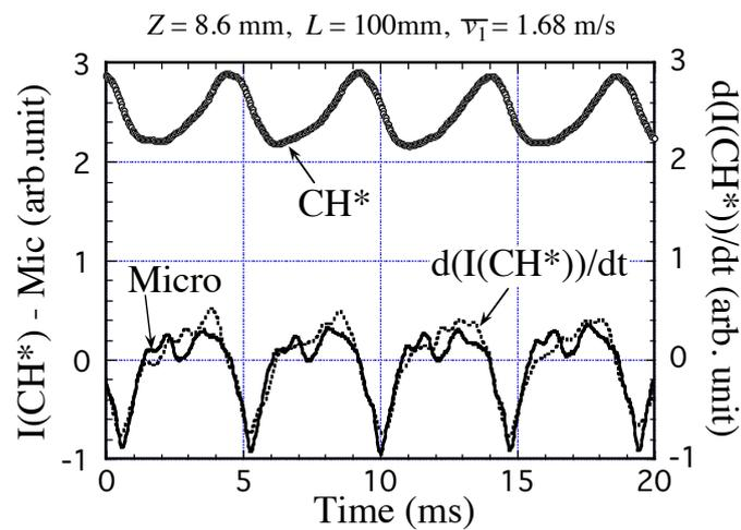
The acoustic pressure and the time derivative of the heat release are similar, confirming that the source is suitably identified
