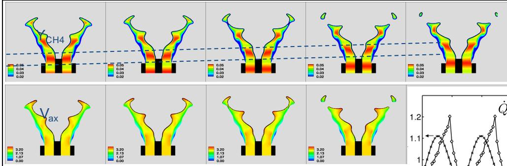
Harmonic mixture composition oscillations are convected and wrinkle the flame (no acoustic forcing):
