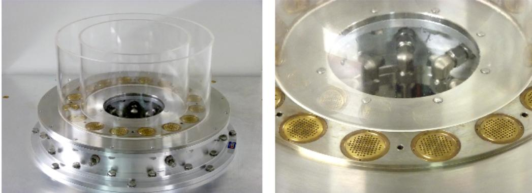
To better understand what determines the structure of the azimuthal modes, it is interesting to work on an annular chamber operating with flames that are simpler than turbulent flames. This is done here by making use of matrix injectors formed by perforated plates
