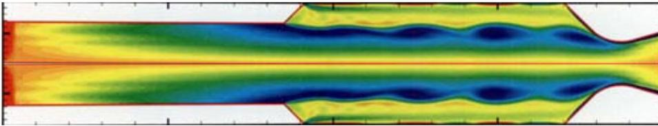
Vortex shedding under controlled operation (pressure fluctuation level is reduced by controller)
