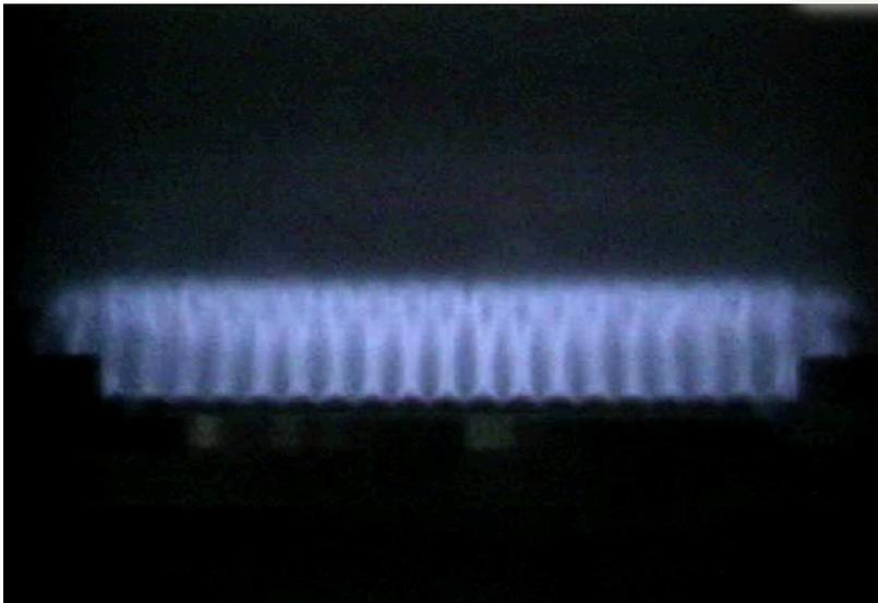
Oscillation cycle ( $f = 530$  Hz) for a typical **unstable combustion regime**.
