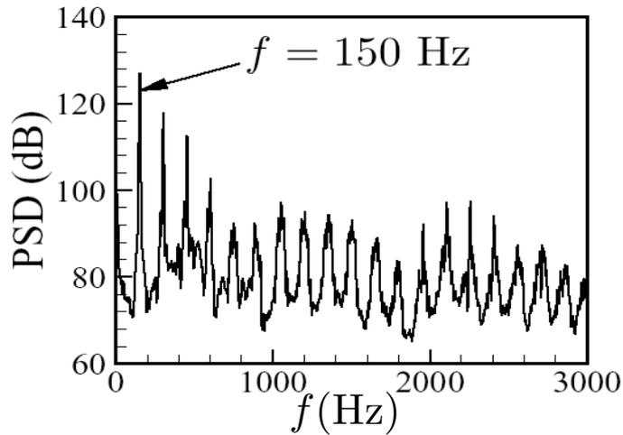
Power spectral density of acoustic pressure during flame/flame interaction
