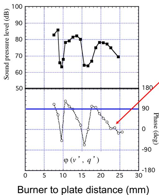
Phase difference between the heat release and the velocity.
