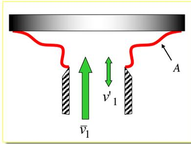
Velocity perturbations are convected by the mean flow along the flame front.
