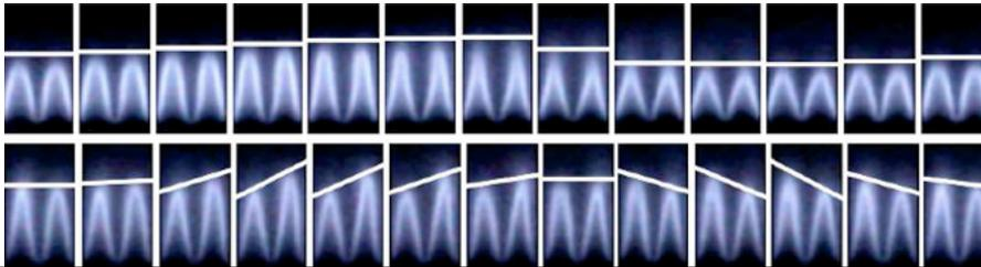
Top : coherent flame response to incoming perturbations. Bottom : response of the system equipped with the DPC
