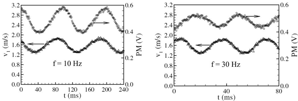
The velocity input is harmonic and the flame response (heat release rate fluctuation) remains also harmonic at these two forcing frequencies
