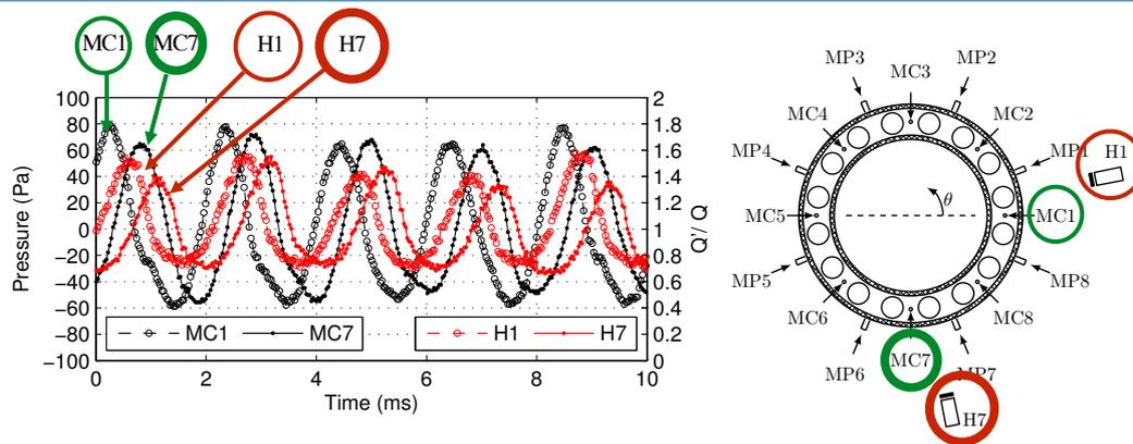
Pressure and photomultiplier signals corresponding to a spinning mode for a bulk velocity  $u_b = 1.49 \text{ m.s}^{-1}$  and an equivalence ratio  $\phi = 0.96$ .
