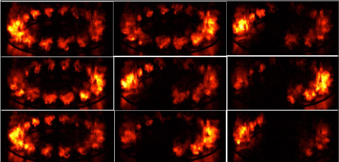
Partial flame blow off in MICCA-Spray in the presence of an azimuthal standing mode of high amplitude (4000 Pa peak)
