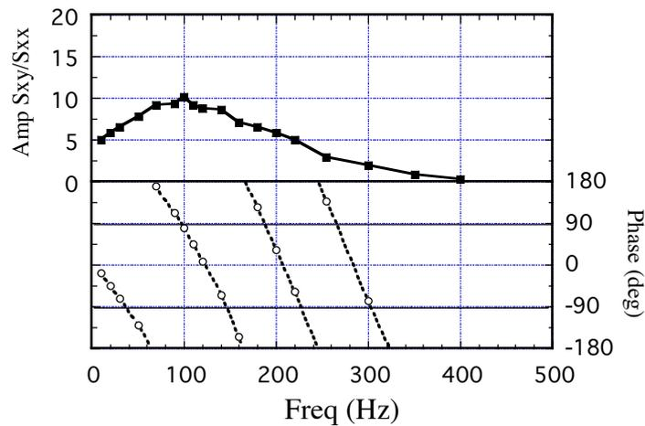
The phase difference between the velocity and the heat release yields a mean convective time which is of the order of  $z/v_1$
