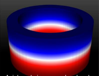
Axial mode in an annular chamber
