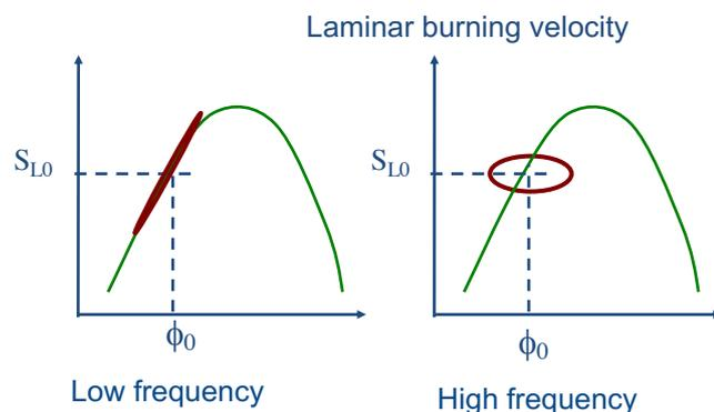
The burning velocity describes (twisted) cycles around steady conditions for increasing modulation frequencies
