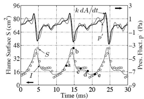
(c) VF :  $f_e = 100 \text{ Hz}$ ,  $\bar{v} = 2.3 \text{ m s}^{-1}$ ,  $v_{rms} = 0.6 \text{ m s}^{-1}$ ,  $\Phi = 1.11$
