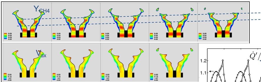
Harmonic mixture composition oscillations are convected and wrinkle the flame (no acoustic forcing):
