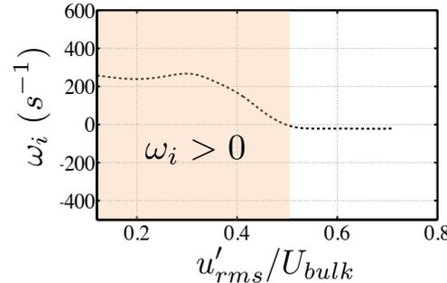
Limit cycle is reached when  $\omega_i$  equals zero. The method yields the limit cycle oscillation level and oscillation frequency.
