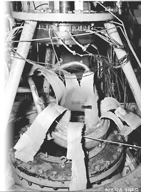
Liquid rocket engine after HF instability
