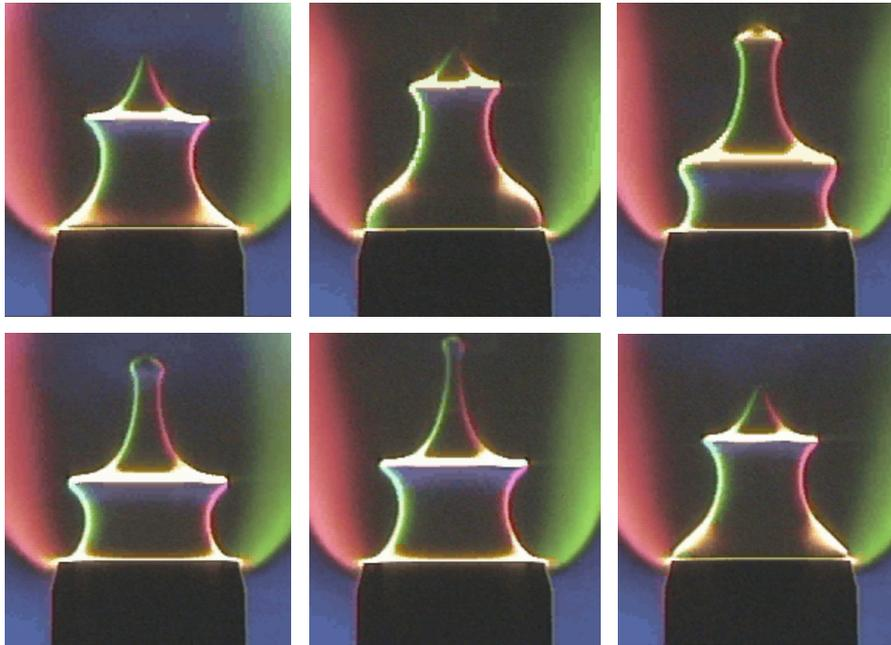
Premixed conical flame submitted to velocity modulations at 75 Hz
