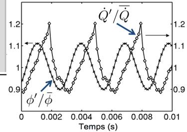
Result in large heat release rate oscillations (nonlinear)
