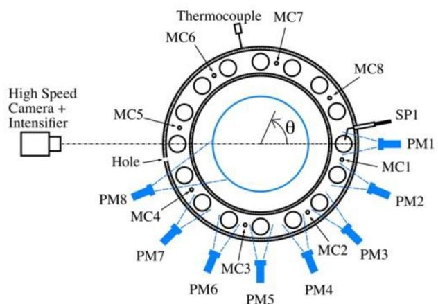
Schematic top view showing locations of the photomultiplier and chamber microphone arrays
