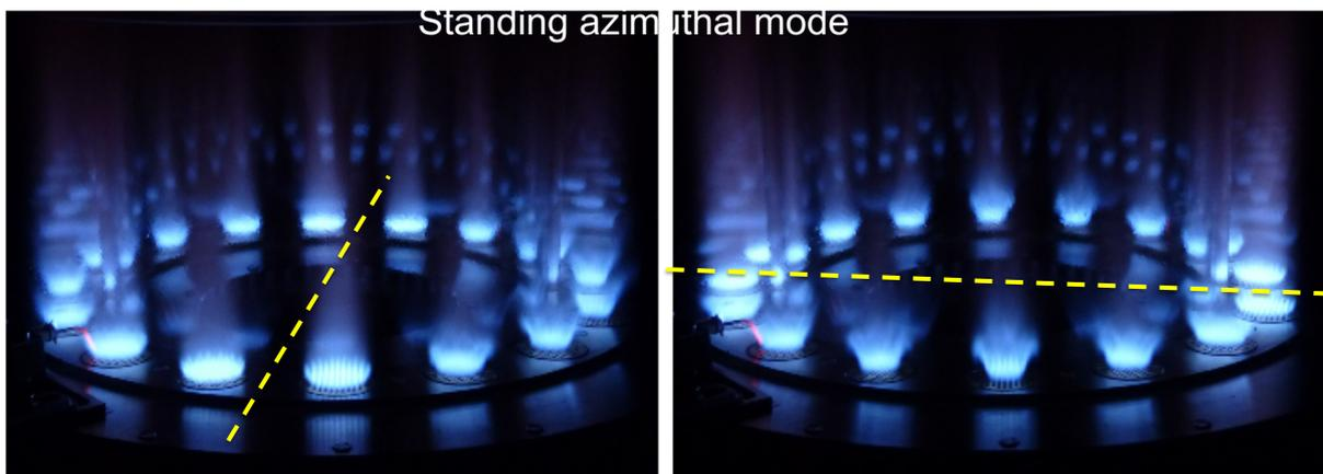
$$v_0 = 2.12 \text{ m s}^{-1} \phi = 1.11$$
