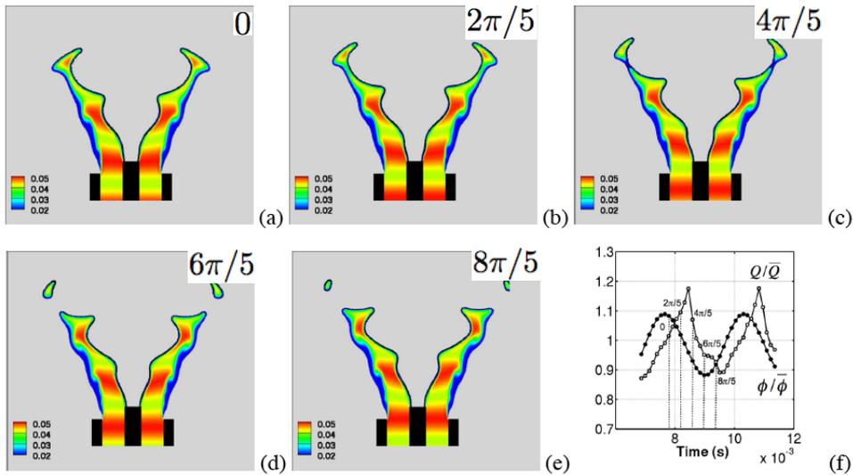
(a-e) Methane mass fraction distributions during a cycle.  $\phi(t) = \phi_0 + \phi_1 \sin \omega t$
