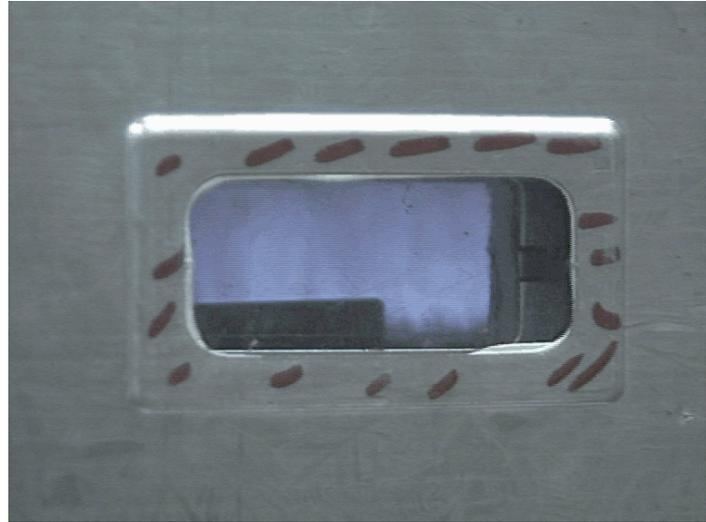
During unstable regime, walls are “breathing” highlighting large pressure oscillations within the combustion
