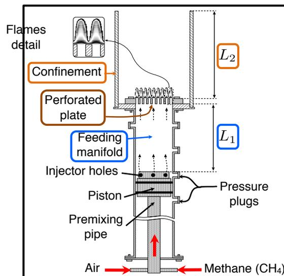
Flexible configuration offering possibilities to analyze combustion instabilities with and without confinement tube
