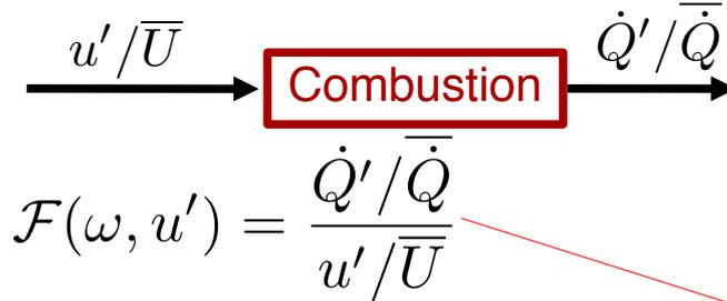
The Flame Describing Function (FDF) extends the transfer function concept to the nonlinear case
