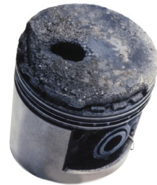
This photo of a badly damaged piston indicates the effects of long-term engine knock.
