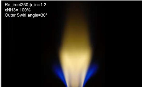
Direct imaging of swirl flame: Effect of xNH<sub>3</sub> on NO emissions at Re<sub>out</sub>=4350, Re<sub>in</sub>=4250,  $\phi_{out}$ =0.7, and  $\phi_{in}$ =1.2
