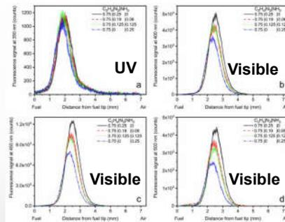
PAH-LIF signal in laminar counter-flow flame.
