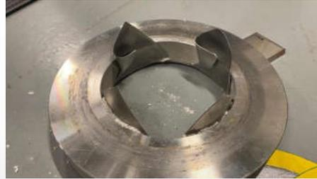
Spec. min at atmospheric pressure was 41.5 bar
