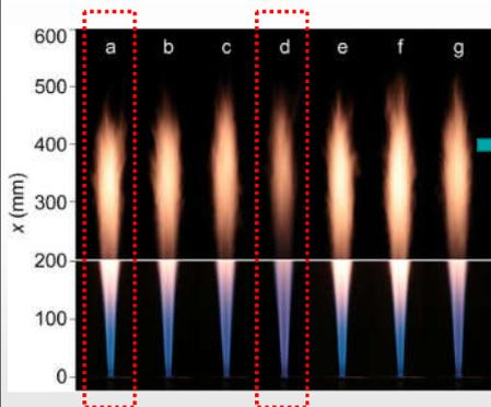
The substitution of ammonia for nitrogen has a noticeable effect on the color of the base of the flame, going from bright blue with no ammonia to dark violet with 25% ammonia.
