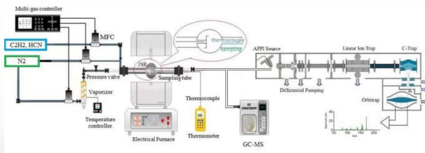
Schematic of apparatus for JSR experiments.
