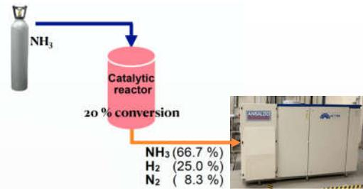
Example of implementation for a 20% NH<sub>3</sub> cracking target
