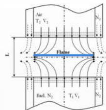
Schematic of a counterflow flame
