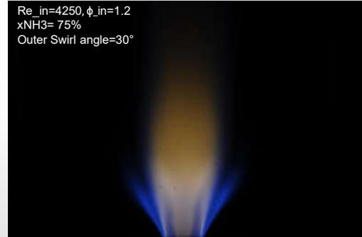
Direct imaging of swirl flame: Effect of xNH<sub>3</sub> on NO emissions at Re<sub>out</sub>=4350, Re<sub>in</sub>=4250,  $\phi_{out}$ =0.7, and  $\phi_{in}$ =1.2
