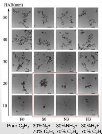
Soot morphology evolution along the centerline of C<sub>2</sub>H<sub>4</sub>/NH<sub>3</sub>/H<sub>2</sub> flames.
