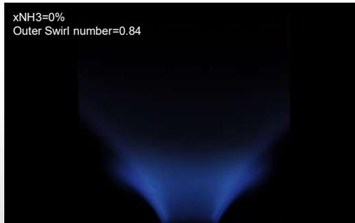
Direct imaging: Effect of outer swirl on the emissions, pure CH<sub>4</sub> in both annuli at  $Re_{out}=4350$ ,  $\phi_{out}=0.7$ ,  $Re_{in}=4250$ ,  $\phi_{in}=1.4$ , and inner swirl number=0.72
