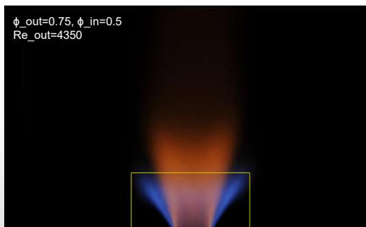
Direct imaging: Outer annulus stream equivalence ratio increased from 0.7 to 0.75 to observe flame stability at Re<sub>out</sub>=4350,  $\phi_{out}$ =0.75, Re<sub>in</sub>=4250, and  $\phi_{in}$ =0.5
