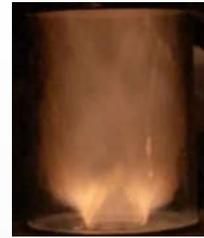
Lean ( $\phi = 0.6$ )  $0.7\text{NH}_3\text{-}0.3\text{H}_2$ -air flame at 4.5 bar
