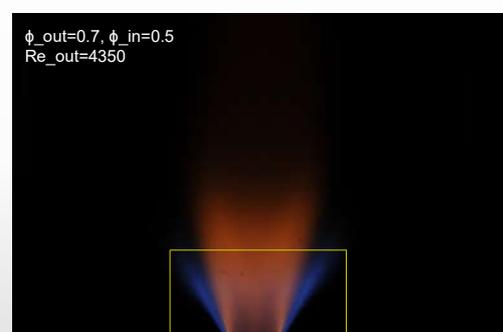
Direct imaging: Outer annulus stream kept at Re<sub>out</sub>=4350,  $\phi_{out}$ =0.7, Re<sub>in</sub>=4250, and  $\phi_{in}$ =0.5
