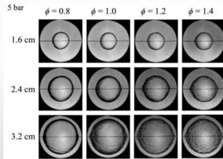
Fig. 11. Images of 2-butanone-air flames with varying equivalence ratios under 423 K and 5 bar.
