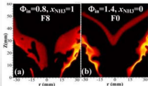
Direct imaging of OH distribution:  $\phi_{\text{out}}$  kept constant (0.6) to observe OH distribution at  $\text{Re}_{\text{out}}=4350$ ,  $\text{Re}_{\text{in}}=4250$ ,  $\phi_{\text{out}}=0.6$ , and  $\phi_{\text{in}}=0.8$ , and  $\phi_{\text{in}}=1.4$
