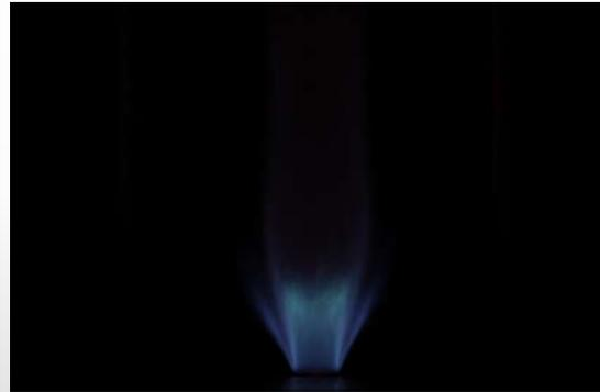
Direct imaging of swirl flame:  $x_{\text{NH}_3}$  increases from 0 to 1 at  $\text{Re}_{\text{out}}=4350$ ,  $\phi_{\text{out}}=0.7$ ,  $\text{Re}_{\text{in}}=4250$ ,  $\phi_{\text{in}}=1.2$ , outer swirl number=0.49, and inner swirl number=0.72
