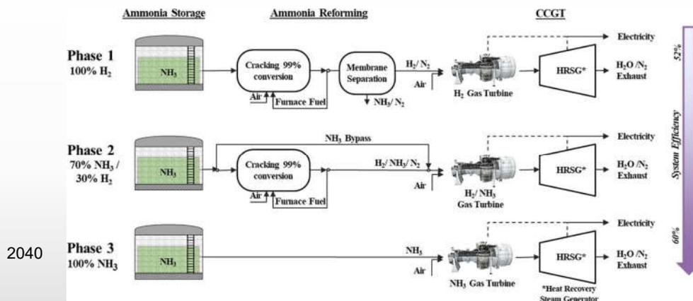
Ammonia fueled CCGT configurations as modelled in three cases of 100% H<sub>2</sub>, 70% NH<sub>3</sub> / 30% H<sub>2</sub>, and 100% NH<sub>3</sub>
