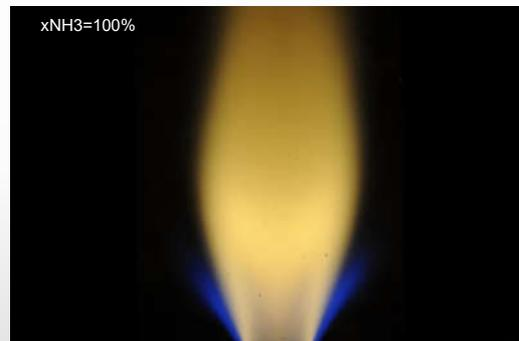
Direct imaging of swirl flame: Inner annulus is pure  $NH_3$ , and outer annulus is pure  $CH_4$  at  $Re_{out}=4350$ ,  $\phi_{out}=0.7$ ,  $Re_{in}=4250$ , and  $\phi_{in}=1.4$
