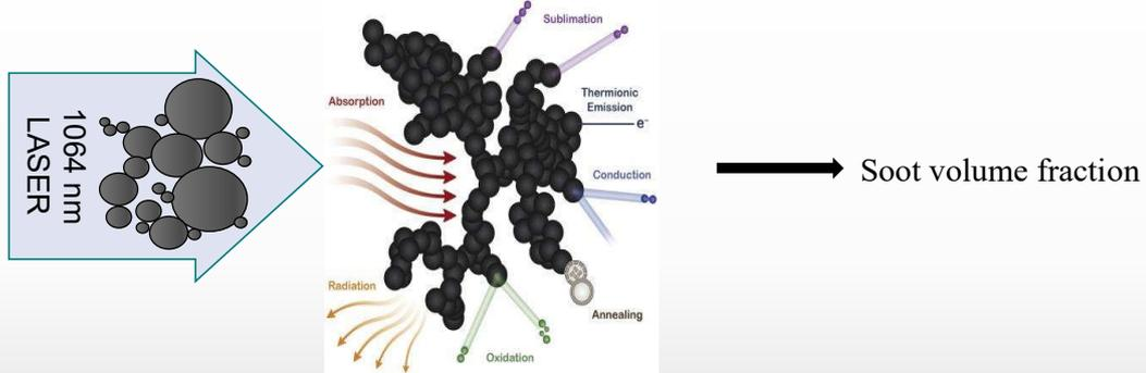
Principle: A short, energetic laser pulse is used as the illumination source. The illuminated soot particles absorb the light and are heated up by the laser pulse to very high temperatures (~4000 K).
