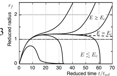
Dynamical quenching of flame kernels in nonflammable mixtures for  $\text{Le} < 1$
