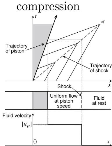
shock wave at constant velocity  $>$  piston velocity
