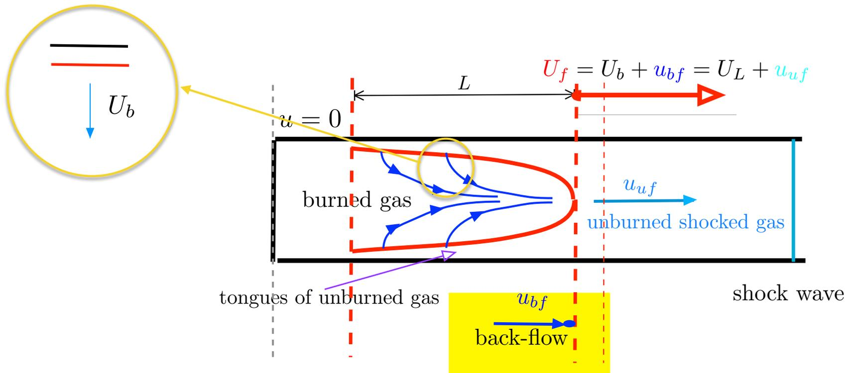
The back flow of burned gas towards the flame tip is well documented
