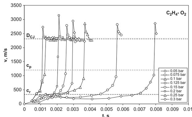
Fig. 6. Velocity-time dependence during detonation initiation in ethylene-oxygen mixture.
