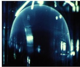
Propane flame propagating upwards
