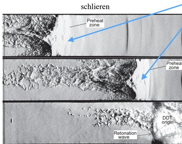
Fig. 7. Sequence of shadow photographs during the second stage and the transition to detonation in ethylene-oxygen mixture,  $P_0=0.12$  bar. Time for the frames from the top is  $t=3.75, 3.85,$  and  $3.95$  ms.
