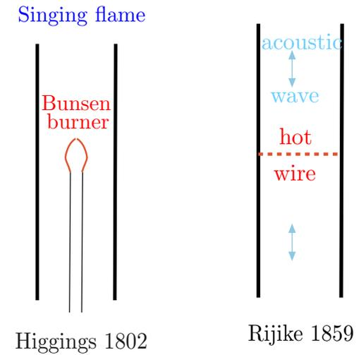
Simplest retro-action mechanism: pressure coupling + 1-D geometry
