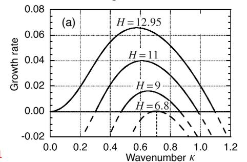
The multidimensional instability develops at a **finite wave length** (larger than the detonation thickness by a factor  $(M_u^2 - 1)^{-1/2}$ ) when increasing the **thermal sensitivity**  $\beta_N$  or the **induction length**  $n$ . The Poincaré-Andronov (Hopf) **bifurcation**
