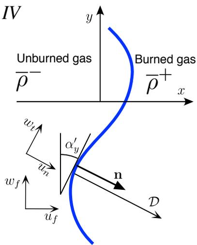
equation of the perturbed front  $x = \alpha(y, t)$  (reference frame !)
