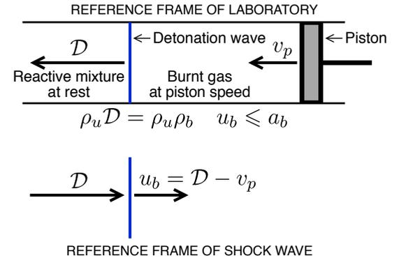
reference frame of **the lead shock wave**
