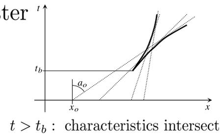
$t > t_b$  : multivalued solution. Wave breaking
