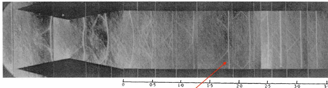
FIGURE 6 (plate 1). Photographs of shock wave at  $M_s = 1.41$ .
