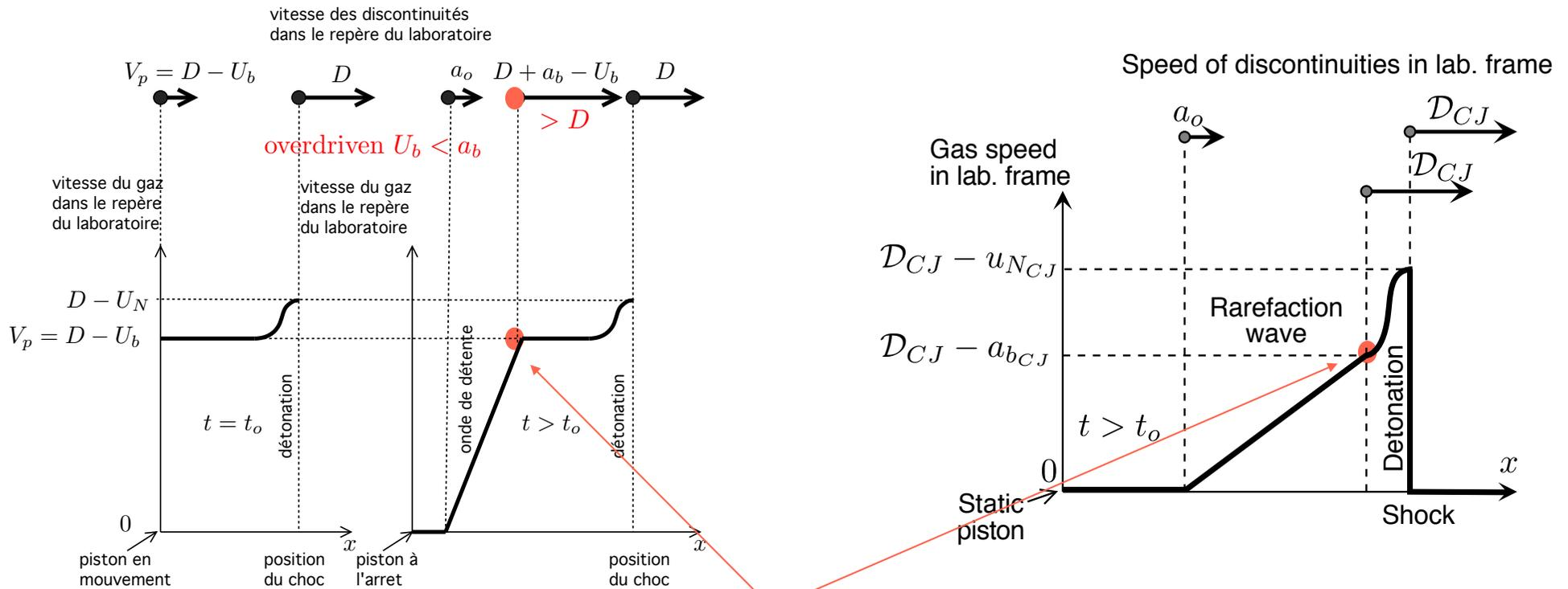
leading edge of the rarefaction wave = speed of sound / gas flow
