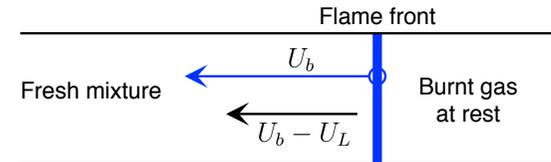
”instantaneous” modification of the flow field, both upstream and downstream
