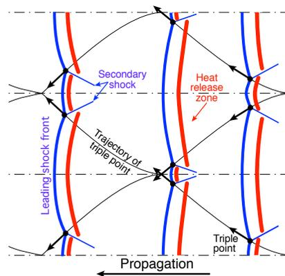
Mach stems propagating in the transverse direction
