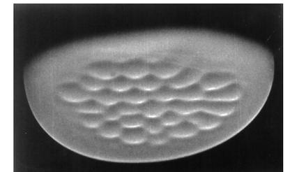
Flames propagating upwards: bubble flames
