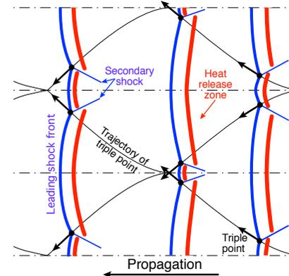
Mach stems propagating in the transverse direction
