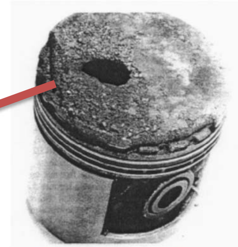
piston damaged by strong knock (LLNL)
