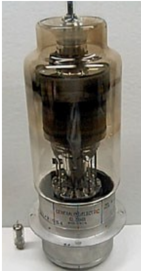
Thyatron (gas-filled tube) High-power electrical switch
