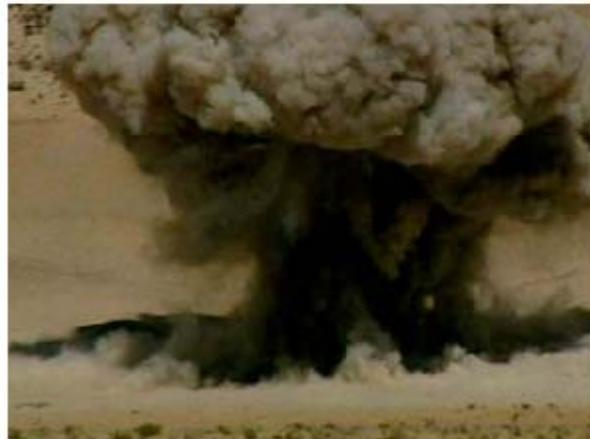
Fig. 3. Open detonation of TNT. Upper figure shows ignition and early burn, lower figure shows entrained cloud of dirt and soot.
