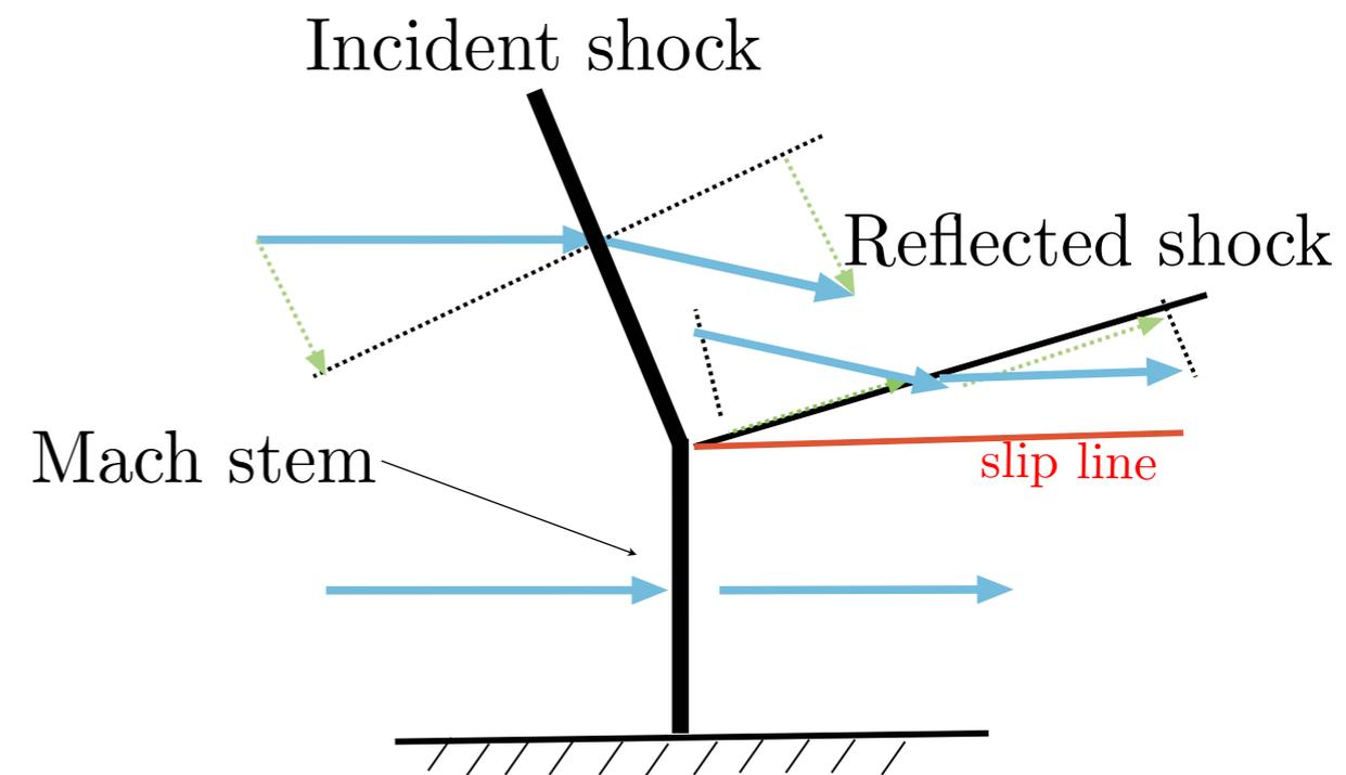
example of a triple point propagating in a uniform flow
