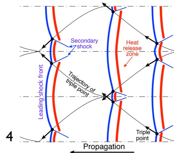
Mach stems propagating in the transverse direction
