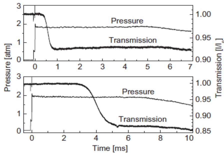
Fig. 1. Typical pressure and laser transmission histories in reflected-shock experiments: (a. upper) 0.1% O<sub>2</sub>, 0.9% H<sub>2</sub>, 99% Ar, 1472 K, 1.83 atm; (b. lower) 0.1% O<sub>2</sub>, 2.9% H<sub>2</sub>, 97% Ar, 1100 K, 1.95 atm.
