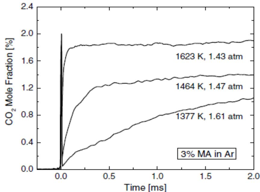
Fig. 3. Measured CO<sub>2</sub> time-histories behind reflected shock waves ( $T_5$ ,  $P_5$  shown) for methyl acetate pyrolysis (3% MA in Ar).
