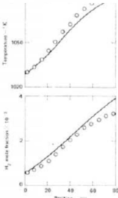
FIGURE 3 Lean flow reactor results using the detailed mechanism from Table I.
