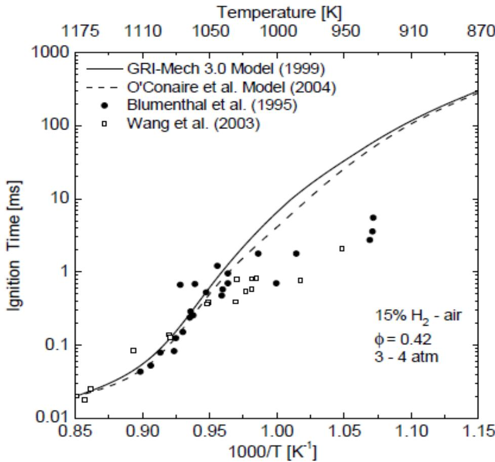
Fig. 1. Reflected-shock ignition delay time data compared to current kinetic models.
