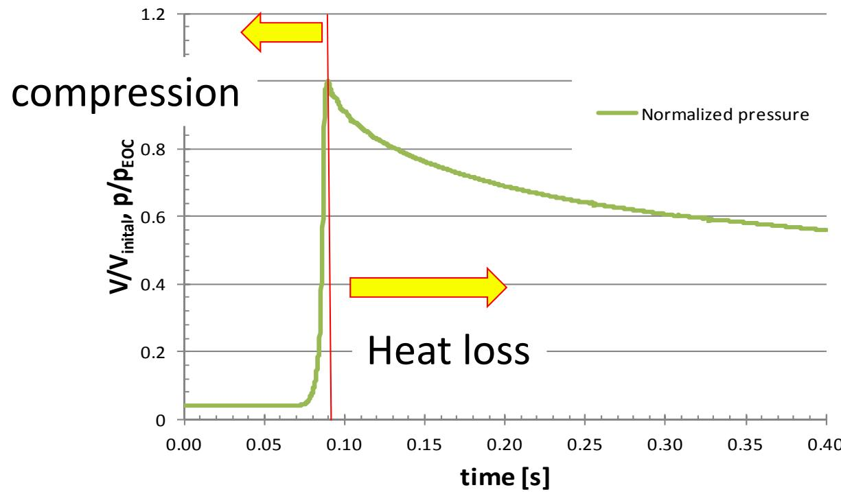
Experiment where  $O_2$  is replaced by  $N_2$  to characterize the compression and heat loss for a specific mixture
