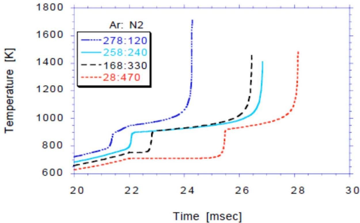
Figure 1. Computed temperature histories for four n-heptane/O<sub>2</sub>/Ar/N<sub>2</sub> mixtures. Temperatures at end of compression are 711, 753, 798 and 949 K in order of increasing Ar concentration.
