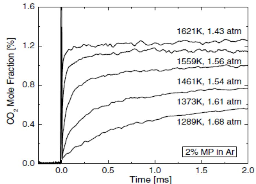
Fig. 4. Measured CO<sub>2</sub> time-histories behind reflected shock waves ( $T_5$ ,  $P_5$  shown) for methyl propionate pyrolysis (2% MP in Ar).
