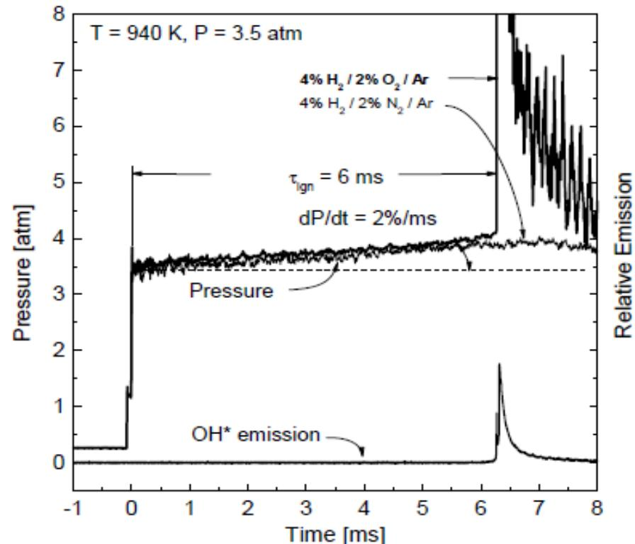
Fig. 2. Experimental data for a 4% H<sub>2</sub>/2% O<sub>2</sub>/Ar test gas mixture at initial post-shock conditions of 940 K and 3.5 atm for reactive and inert mixtures.
