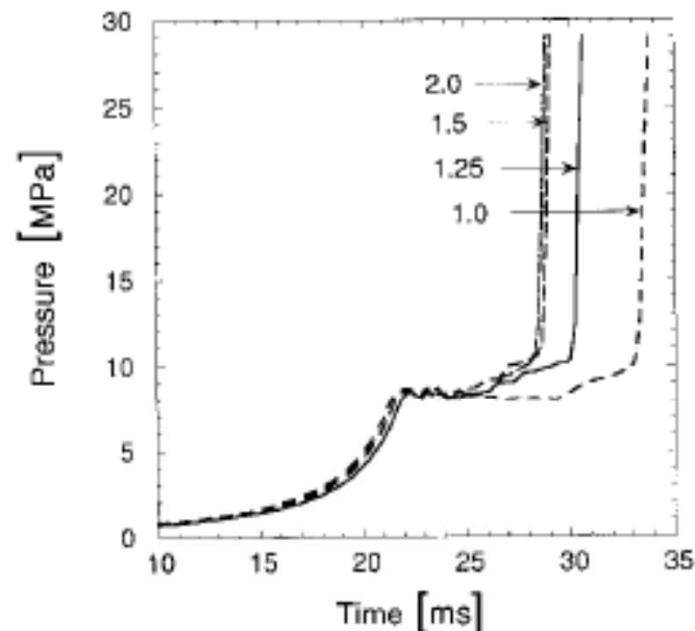
FIG. 3. Experimental pressure records for ignition following compression to 724 ( $\pm 6$  K) at indicated values of equivalence ratio. Initial pressures are all 0.33 bar.
