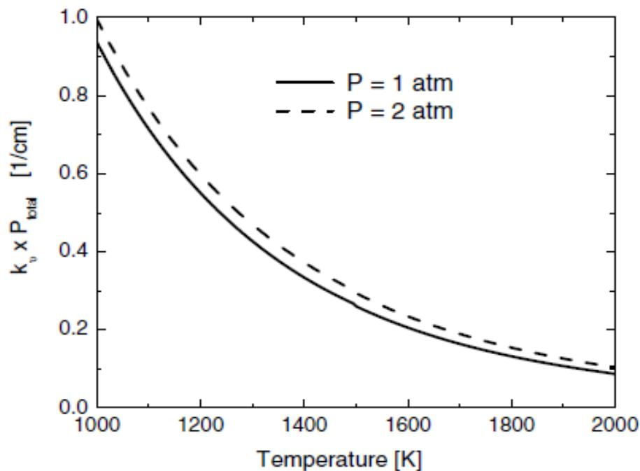
Fig. 1. Absorption coefficient  $\times$  pressure product,  $k_v \times P_{\text{total}} [\text{cm}^{-1}]$  for the R(28)  $\text{CO}_2$  transition near  $3633.08 \text{ cm}^{-1}$  (2752.5 nm) at  $P = 1$  and 2 atm.
