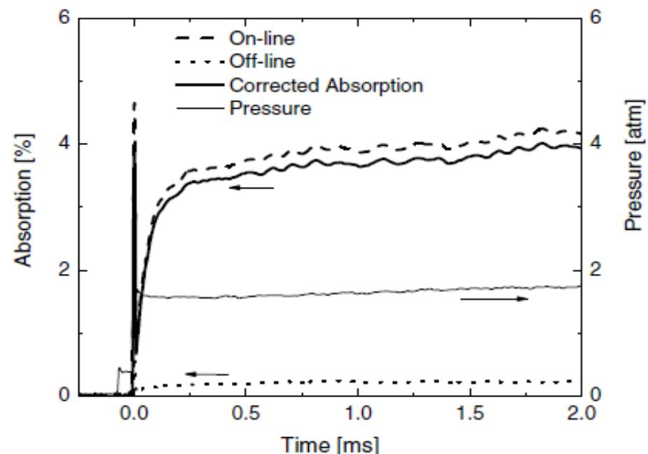
Fig. 2. Example on-line and off-line absorption measurement in 2% MB/Argon. Reflected shock conditions:  $T_5 = 1426 \text{ K}$ ,  $P_5 = 1.58 \text{ atm}$ . On-line wavenumber =  $3633.08 \text{ cm}^{-1}$ ; Off-line wavenumber =  $3633.25 \text{ cm}^{-1}$ .
