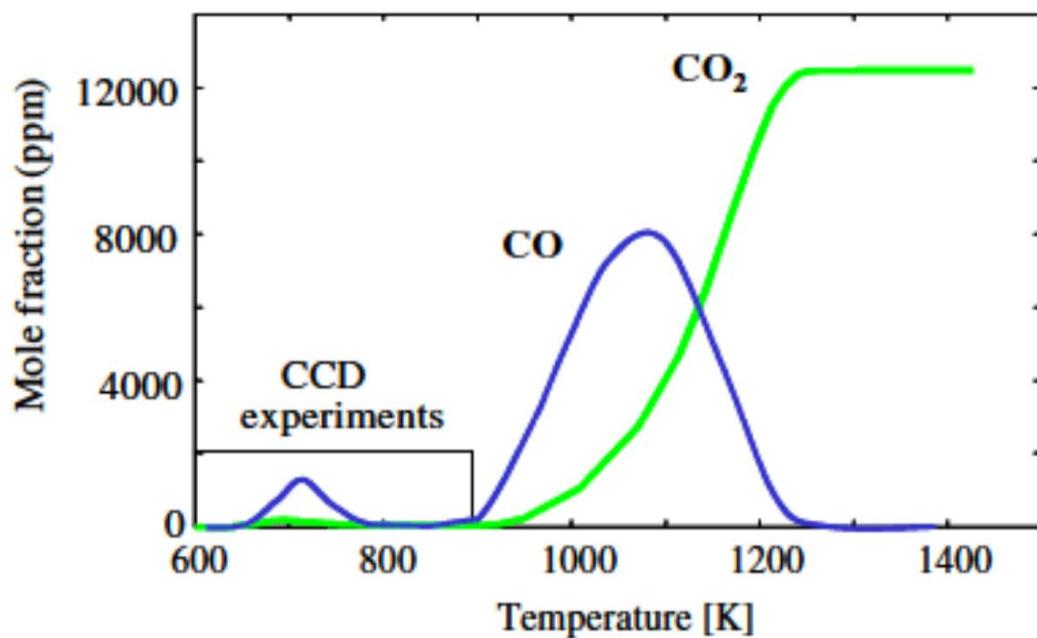
Fig. 2. CO and CO<sub>2</sub> production vs. reactor temperature for *n*-dodecane oxidation (ND1), showing the typical extent of a CCD experiment.
