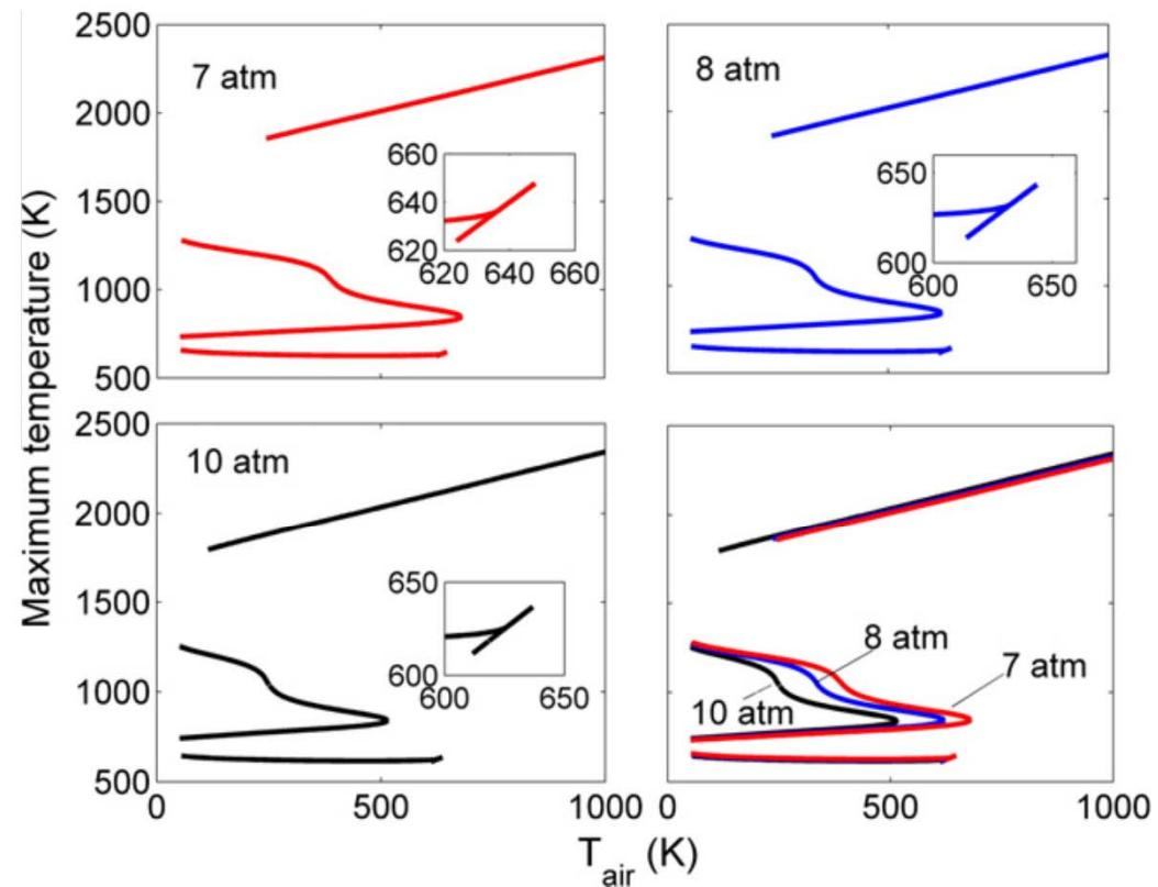
**Fig. 19.** The global response S-curve of the diffusion counterflow: maximum temperature versus air-side boundary temperature from 7 atm to 10 atm, with a pressure-weighted strain rate 100 (1/s).
