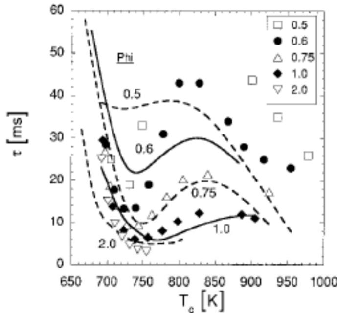
FIG. 4. Variations in total ignition delay time with compression temperature for selected values of equivalence ratio. Curves represent fits to experimental results and are labeled by the value of the equivalence ratio, symbols indicate computed results for values of  $\phi$  shown in the legend. Initial pressures are all 0.33 bar.
