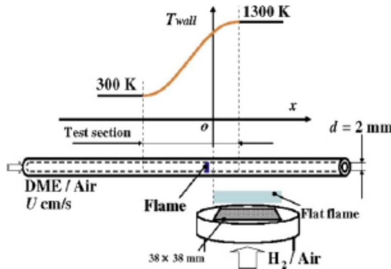
Fig. 13. A narrow channel with a prescribed wall temperature profile. Inner diameter of 2 mm, which is smaller than the ordinary quenching diameter, was chosen. Though hydrogen/air flat flame burner was shown as a heat source here, flat panel heaters were also used for earlier study.
