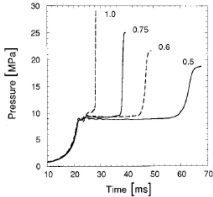
FIG. 2. Experimental pressure records for ignition following compression to 765 ( $\pm 5$  K) at indicated values of equivalence ratio. Initial pressures are all 0.33 bar.
