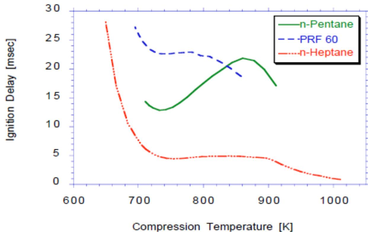
Figure 3. Computed ignition delay times, including reaction during compression stroke, for n-heptane, n-pentane, and PRF 60 mixture.
