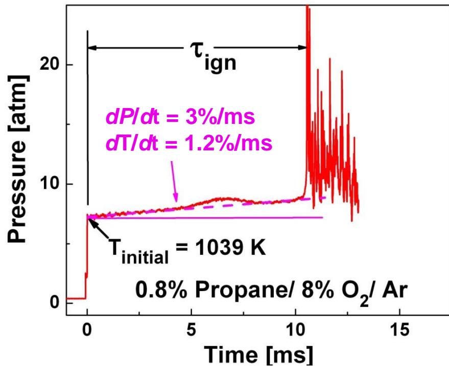
Shock Tubes are ideal for measuring homogeneous gas phase reaction kinetics
