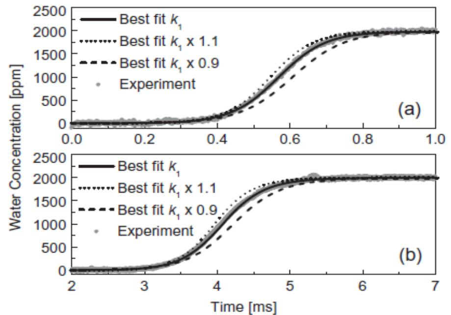
Fig. 3. Comparison of experimental and Senkin calculated H<sub>2</sub>O profiles using best-fit  $k_1$  with effect of  $\pm 10\%$  variation on  $k_1$  at conditions of the corresponding panels of Fig. 1.
