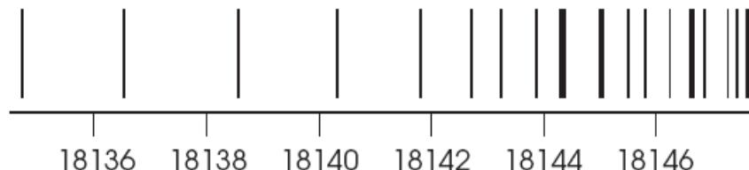
Rotational spectrum in the 0-0 band of an electronic transition ( $A^3\Pi_{0+u} - X^1\Sigma_g^+$ ) in  $^{35}\text{Cl}_2$
