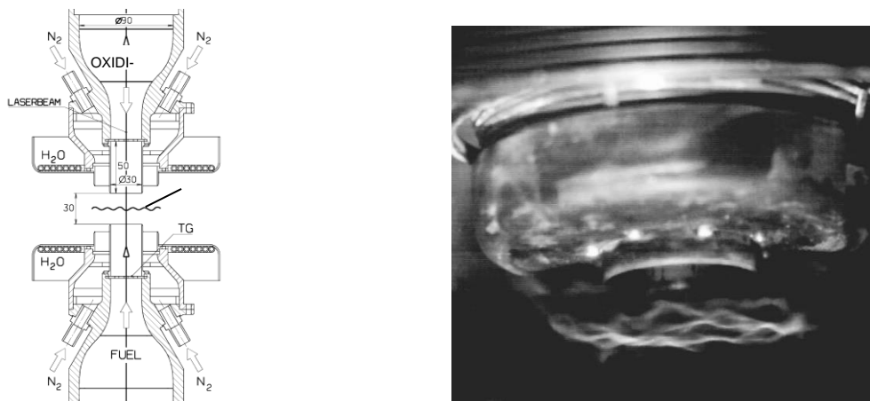
Figure 2.1 Schematic of the turbulent opposed jet burner (left) and snapshot of the luminous flame using a CMOS-camera operated with an exposure time of 2ms.
